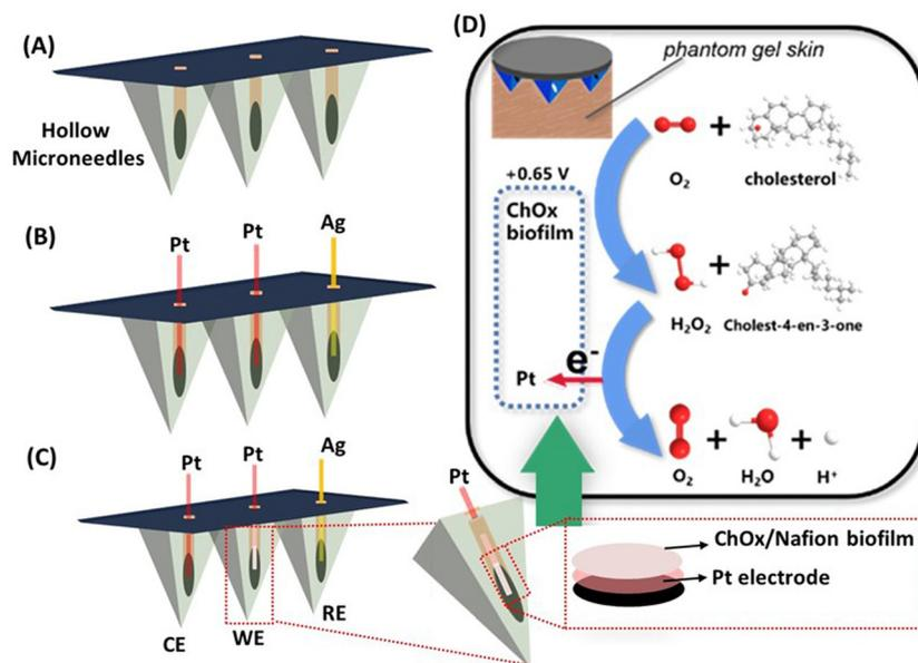
Fig. 1 Schematic illustration of (A) the hollow microneedle, (B) Pt and Ag wires integrated with the microneedle array, (C) ChOx/Nafion functionalization of the Pt electrode, and (D) the reaction mechanism associated with the minimally invasive wearable microneedle sensor for the detection of cholesterol.
