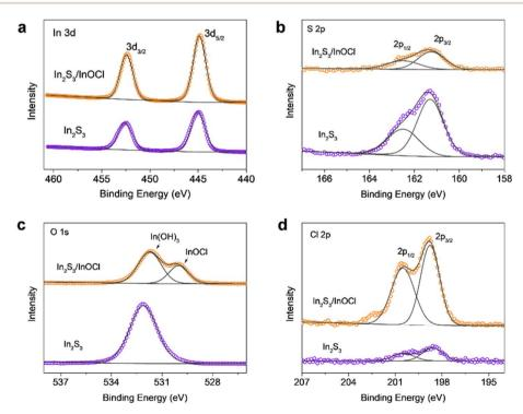
Fig. 2 XPS spectra of (a) In 3d, (b) S 2p, (c) O 1s, and (d) Cl 2p of In<sub>2</sub>S<sub>3</sub> buffer layers without and with the InCl<sub>3</sub> post-treatment.
