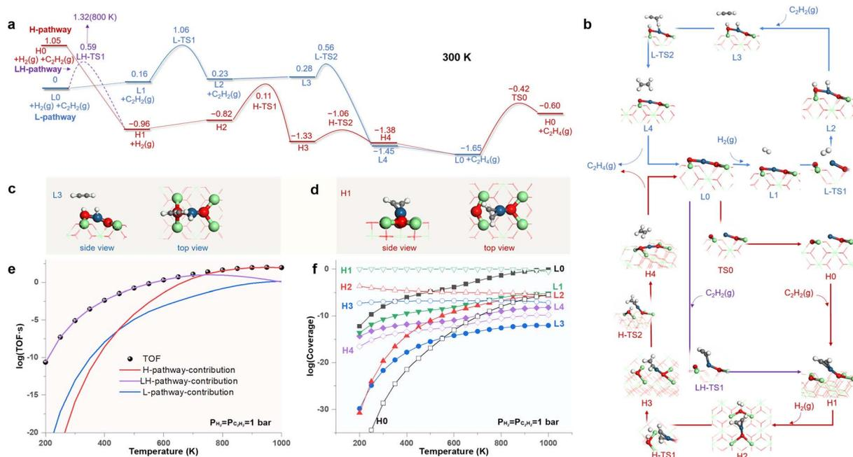
Fig. 4 (a) Free energy profiles (in eV) of SHA on the  $\text{Pt}_1/\text{CeO}_2$  SAC following pathways enabled by the LES (L-pathway) and the HEMS (H-pathway). (b) Structures of all states. Configurations of  $\text{C}_2\text{H}_2$  activation on (c) the LES and (d) the HEMS. Calculated (e) turnover frequency (TOF) and (f) coverages of states as functions of temperature.
