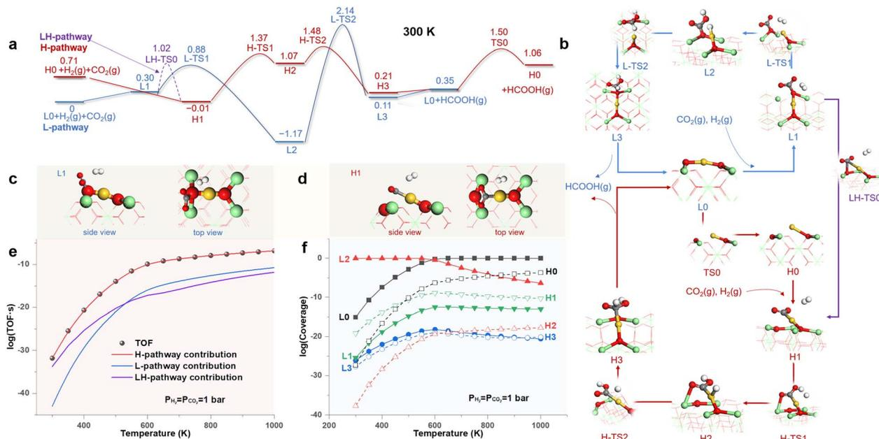
Fig. 3 (a) Free energy profiles (in eV) of  $\text{CO}_2\text{HR}$  on the  $\text{Au}_1/\text{CeO}_2$  SAC following pathways enabled by the LES (L-pathway) and HEMS (H-pathway). (b) Structures of all states. Configurations of  $\text{CO}_2$  activation on (c) the LES and (d) the HEMS. Calculated (e) turnover frequency (TOF) and (f) coverages of states as functions of temperature.
