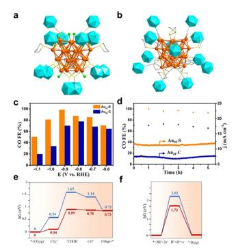
Fig. 11 The total structures of (a)  $Au_{28}(C_2B_{10}H_{11}S)_{12}(tht)_4Cl_4$  and (b)  $[Au_{28}(C_4B_{10}H_{11})_{12}(tht)_8]^{3+}$ . (c) Faradaic efficiency of CO and (d) stability testing of two nanoclusters. Free energy of (e) eCO2RR and (f) HER on  $Au_{28}(C_2B_{10}H_{11}S)_{12}(tht)_4Cl_4$  (red) and  $[Au_{28}(C_4B_{10}H_{11})_{12}(tht)_8]^{3+}$  (blue). Copyright 2022, Wiley.<sup>97</sup>
