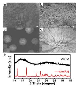
Fig. 5 SEM images of Au-PA precursors at (a) 5  $\mu$ m, (b) 500 nm and (Au-PA)<sub>f</sub> precursors at (c) 5  $\mu$ m, (d) 500 nm. (e) XRD patterns of the amorphous Au-PA precursor generated without ethanol and the flower-like (Au-PA). precursor generated with the presence of ethanol. Copyright 2020, Royal Society of Chemistry.54
