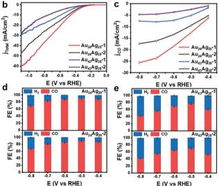
Fig. 13 (a) Structural anatomy of four nanoclusters. (b) LSV curves and (c) the corresponding CO partial current density of the  $Au_{24}Ag_{20}$  and  $Au_{43}Ag_{38}$  nanoclusters. Faradaic efficiency for  $CO_2RR$  products obtained on (d)  $Au_{24}Ag_{20}$  and (e)  $Au_{43}Ag_{38}$  nanoclusters. Copyright 2022, Royal Society of Chemistry.<sup>75</sup>
