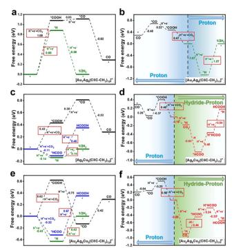
Fig. 10 Free energy of eCO<sub>2</sub>RR and HER on (a) and (b) intact and incomplete  $Au_7Ag_8$ , (c) and (d)  $Ag_9Cu_6$  and (e) and (f)  $Au_2Ag_8Cu_5$ . Copyright 2022, Royal Society of Chemistry. 95
