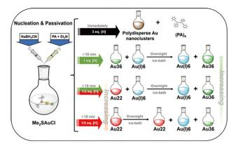
Fig. 6 Synthetic routes for Au<sub>36</sub>(PA)<sub>24</sub> with the different amounts of reducing agents in the synchronous nucleation and passivation strategy. Copyright 2020, Springer. 47
