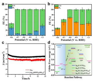
Fig. 12 Faradaic efficiency of CO for (a)  $Ag_{32}(C \equiv CAr^F)_{24}$  and (b)  $[Ag_{32}(DPPE)_5(SR)_{24}]^2$  at different potentials. (c) Stability testing of two nanoclusters. (d) Comparison of  $\Delta G$  of  $eCO_2RR$  on  $Ag_{32}(C \equiv CCH_3)_{24}$ .  $Ag_{32}(C \equiv CCH_3)_{23}$ ,  $[Ag_{32}(P_2C_2H_6)_5(SCH_3)_{24}]^2$  and  $[Ag_{32}(P_2C_2H_6)_5(SCH_3)_{23}]^2$  with the HER. Copyright 2022, Springer.<sup>37</sup>
