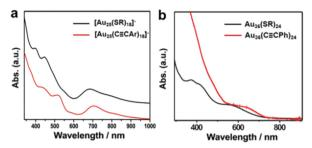
Fig. 3 The comparison of optical properties of (a) [Au<sub>25</sub>(PhC≡CAr)<sub>18</sub>]<sup>-</sup>,  $[Au_{25}(SR)_{18}]^{-}$  and (b)  $Au_{36}(PhC \equiv C)_{24}$ ,  $Au_{36}(SR)_{24}$ . Copyright 2017 and 2018, Wiley. 38,39
