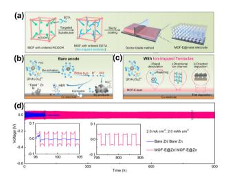
**Fig. 7** (a) Schematic of ordered HCOOH in MOF-808 be substituted by EDTA to form MOF-808 with ordered EDTA (MOF-E) and the process of electrode preparation. Schematic of Zn deposition on (b) bare Cu and (c) MOF-E@Cu. (d) Zn plating/stripping in a symmetric cell with MOF-E@Zn and bare Zn. Reproduced from ref. 69 with permission from John Wiley & Sons, copyright 2023.
