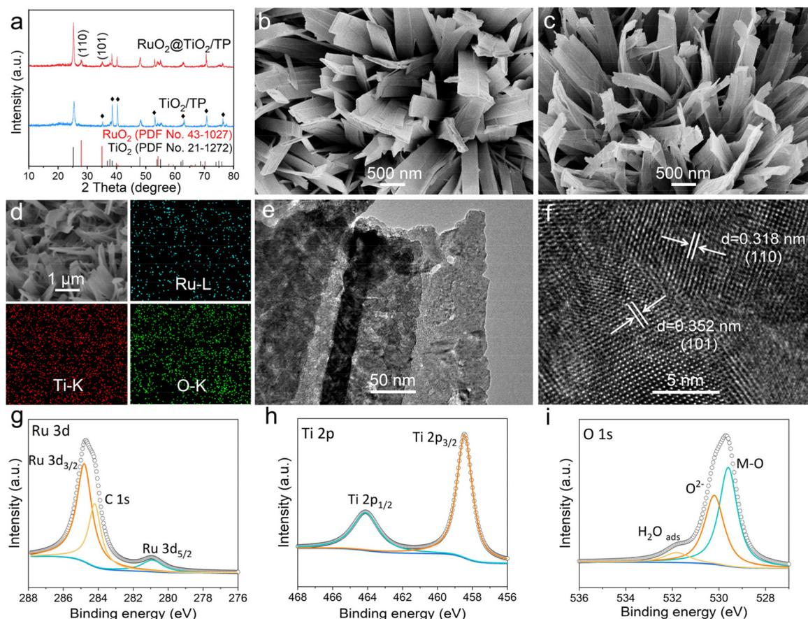
**Fig. 1** (a) XRD patterns of  $\text{RuO}_2@\text{TiO}_2/\text{TP}$  and  $\text{TiO}_2/\text{TP}$ . SEM images of (b)  $\text{TiO}_2/\text{TP}$  and (c)  $\text{RuO}_2@\text{TiO}_2/\text{TP}$ . (d) The SEM image and corresponding EDX elemental mapping images of  $\text{RuO}_2@\text{TiO}_2/\text{TP}$ . (e) TEM and (f) HRTEM images of  $\text{RuO}_2@\text{TiO}_2$ . High-resolution XPS spectra of  $\text{RuO}_2@\text{TiO}_2/\text{TP}$  in (g) the Ru 3d, (h) the Ti 2p, and (i) the O 1s regions.
