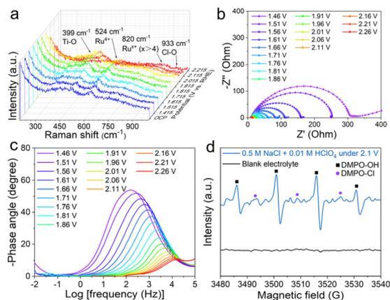
**Fig. 3** (a) *In situ* Raman spectra recorded for RuO<sub>2</sub>@TiO<sub>2</sub>/TP, shown as a function of potential, during the CER in 6 M NaCl + 0.01 M HClO<sub>4</sub>. (b) Nyquist plots and (c) Bode phase plots for RuO<sub>2</sub>@TiO<sub>2</sub>/TP at different applied potentials in 0.5 M NaCl + 0.01 M HClO<sub>4</sub>. (d) Quasi *in situ* EPR trapping of the radicals.
