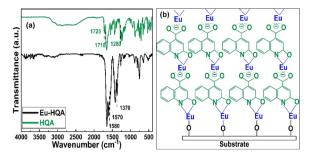
Fig. 3 (a) FTIR spectra for HQA precursor powder and a representative Eu-HQA thin film sample. (b) Schematics of the anticipated film growth mode/bonding scheme in our Eu-HQA films.
