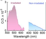
Fig. 4 Detection of iron ions. (A) Scheme of the purification process and the metal complex used for detecting the presence of released iron ions. Irradiated NFs (or non-irradiated for control) were filtered, and the filtrate was treated with 1,10-Phenanthroline (phen), resulting in the orange-red metal complex [Fe(phen)<sub>3</sub>]<sup>2+</sup>. (B) Extinction spectra obtained from the filtrates of NF dispersions without (blue) and with (magenta) 808 nm irradiation (P = 200 mW).
