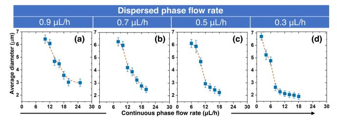
Fig. 4 Relationship between QD-MB diameter and continuous flow rates. The dispersed flow rate was set at 0.9 μL h<sup>-1</sup> (a), 0.7 μL h<sup>-1</sup> (b), 0.5 μL h<sup>-1</sup> (c), and 0.3 µL h<sup>-1</sup> (d). Increasing the continuous flow rate led to a decrease in the average diameter of QD-MBs. The coefficient of variance for the size distribution was less than 10%.
