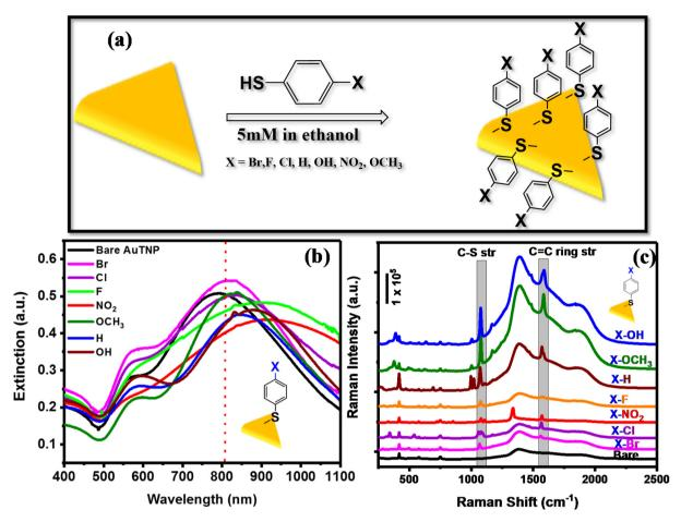
Fig. 2 (a) Schematic representation of the AuTP substrate functionalization with the various *p*-substituted benzene thiol ligands (X-Ph-SH). The figure is not to scale. (b) LSPR spectra of Bare AuTP (black) and after functionalization with different ligands. LSPR peak red-shift observed after each thiol functionalization. (c) SERS analysis of bare AuTP (black) and after functionalization with X-Ph-SH.
