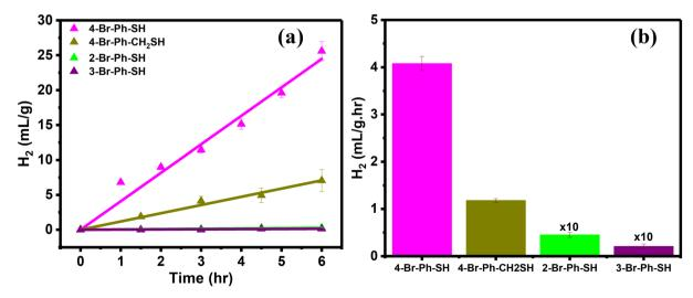
Fig. 4 (a) Photocatalytic  $H_2$  production was observed over time for *ortho-, meta-,* and *para-substituted* benzene-thiols and with 4-Br-Ph-CH<sub>2</sub>-SH functionalized AuTP substrates. (b) Comparison of the  $H_2$  production rate observed with different Br substituted substrates. The experiment was performed in neutral water under 808 nm laser illumination with a 100 mW cm<sup>-2</sup> power density.
