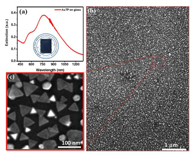
Fig. 1 (a) UV-visible extinction spectra of AuTP attached to the glass substrate. The inset shows the photo of the AuTP functionalized glass substrate. (b) Corresponding SEM image of the AuTP functionalized on ITO substrate. The scale bar is 1  $\mu$ m. (c) The zoom-out SEM image of AuTP. The scale bar is 100 nm.
