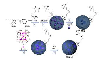
Scheme 1 Schematic representation of the synthesis of functionalized hybrid nanoparticles MSN-1 and MSN-2. The used complexes 1 or 2 are  $[(Tb/Eu)_9(acac)_{16}(\mu_3-OH)_8(\mu_4-O)(\mu_4-OH)]\cdot H_2O$  (where Tb/Eu ratio = 19/1 for 1 and 9/1 for 2).
