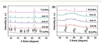
Fig. 7 XRD patterns of (a) Y-phase  $CsPb_xSn_{1-x}I_3$  NWs and (b) B- $\gamma$  phase CsPb<sub>x</sub>Sn<sub>1-x</sub>I<sub>3</sub> NWs. Reproduced from ref. 78 with permission from the American Chemical Society. Copyright 2018.
