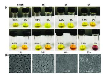
Fig. 6 (a) Photographs of CsPb<sub>0.5</sub>Sn<sub>0.5</sub>I<sub>2</sub>Br precursor solutions with and without TP (0.5%). (b) Top-view SEM images of CsPb<sub>0.5</sub>Sn<sub>0.5</sub>I<sub>2</sub>Br thin films with varing TP contents. Reproduced from ref. 74 with permission from Wiley-VCH. Copyright 2020.
