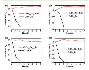
Fig. 8 Stability tests of CsPb<sub>0.8</sub>Ge<sub>0.2</sub>l<sub>2</sub>Br and CsPbl<sub>2</sub>Br PSCs upon the storage in the ambient atmosphere (50--60 % RH): (a)  $V_{OC}$ , (b) FF, (c)  $J_{SC}$ , and (d) PCE. Reproduced from ref. 80 with permission from Wiley-VCH. Copyright 2018.
