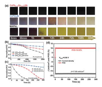
Fig. 4 (a) Photographs of  $CsPb_{0.55}Sn_{0.45}l_2Br$ ,  $CsPbl_2Br$  and  $MAPbl_3$  perovskite films under iso-thermal annealing (150 °C) in an  $N_2$ -filled glove box. The long-term normalized PCE of PSCs (b) in an  $N_2$ -filled glovebox and (c) in the ambient air (40–50% RH). (d) MPPT of a  $CsPb_{0.55}Sn_{0.45}l_2Br$ -CsCl-S-based device. Reproduced from ref. 68 with permission from Wiley-VCH. Copyright 2021.
