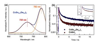
Fig. 11 (a) Steady-state PL spectra of CsSn<sub>0.6</sub>Ge<sub>0.4</sub>I<sub>3</sub> NCs. (b) TRPL spectra of CsSn<sub>0.6</sub>Ge<sub>0.4</sub>I<sub>3</sub> and CsSnI<sub>3</sub>. Reproduced from ref. 86 with permission from Wiley-VCH, copyright 2020.
