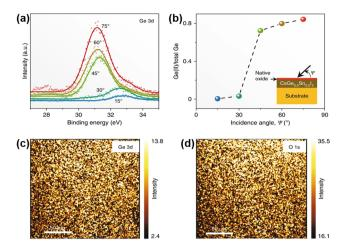
Fig. 10 (a) Ge 3d XPS spectra at different incidence angles in a vapordeposited CsSn<sub>0.5</sub>Ge<sub>0.5</sub>I<sub>3</sub> film. (b) The corresponding plot of the Ge(II) fraction vs. the incidence angle. (c) and (d) XPS maps of Ge 3d (33 eV) and O 1s (532 eV). Reproduced from ref. 82 with permission from Springer Nature. Copyright 2020.
