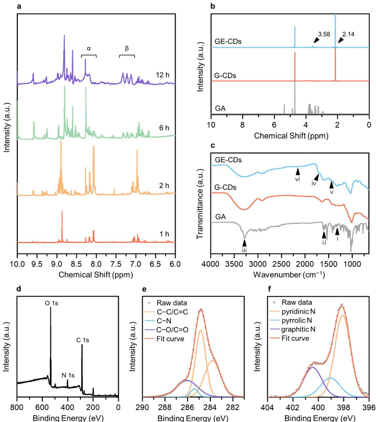
Fig. 1 (a)  $^1\text{H}$  NMR spectra of GE-CDs with different reaction times. (b)  $^1\text{H}$  NMR spectra of GA, G-CDs, and GE-CDs. (c) FTIR spectra of GA, G-CDs, and GE-CDs. (d) XPS spectrum of GE-CDs. High-resolution XPS spectra of (e) carbon 1s and (f) nitrogen 1s of GE-CDs.
