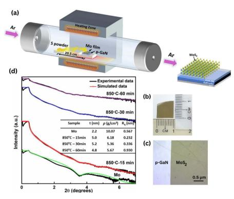
Fig. 1 (a) Schematic illustration of the CVD setup. (b) Photograph image of the MoS<sub>2</sub> film deposited on 1 cm  $\times$  1 cm p-GaN. (c) Optical image of the large-area patterned MoS<sub>2</sub> film grown on p-GaN through a shadow mask, taken at 20× magnification. (d) X-ray reflectivity curve of the asgrown Mo and MoS $_2$  films deposited on p-GaN at 850 °C - 15 min, 850 °C - 30 min and 850 °C - 60 min.
