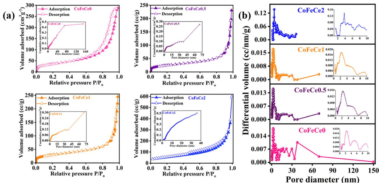
Fig. 4 (a) N<sub>2</sub> adsorption–desorption isotherm profile at 77 K. Insets show the cumulative pore volume of the respective samples, and (b) pore size distribution (inset shows small pore region) of Ce-doped CoFe LDHs.
