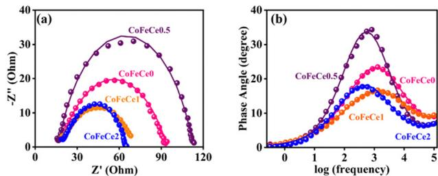
Fig. 8 (a) Nyquist plots, and (b) Bode plots at a bias potential of 1.54 V vs. RHE in the frequency range from  $10^5$  to  $10^{-1}$  s $^{-1}$  with 0.005 V amplitude for different LDHs. The experimental results are represented by discrete points and equivalent circuit fitted results are represented by solid lines.
