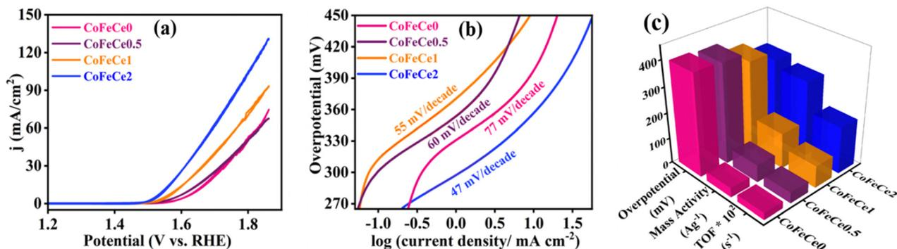
Fig. 6 Electrochemical results of LDHs. (a) CVs at a scan rate of  $5 \text{ mV s}^{-1}$ , (b) Tafel plots of Ce-doped CoFe LDHs during water oxidation and (c) overpotentials, mass activities, and TOFs of the Ce-doped CoFe LDHs during water oxidation. Overpotentials were measured at  $10 \text{ mA cm}^{-2}$  current density. Mass activities and TOFs were calculated at  $350 \text{ mV}$  overpotential.
