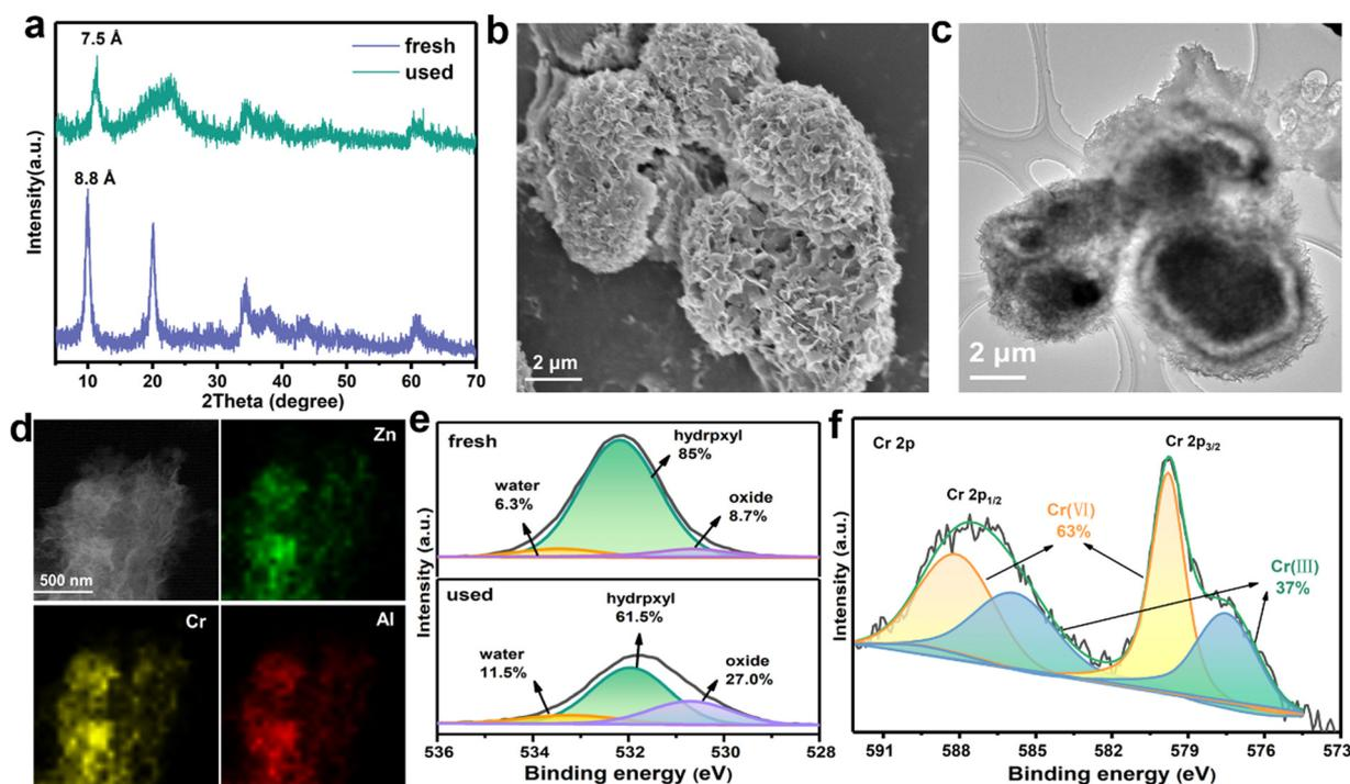
Fig. 5 (a) XRD patterns of ZnAl-LDH-D before and after adsorption of Cr<sup>VI</sup>; (b) SEM image of ZnAl-LDH-D after adsorption of Cr<sup>VI</sup>; (c) and (d) TEM image and the EDS mapping of ZnAl-LDH-D after adsorption of Cr<sup>VI</sup>; (e) high-resolution XPS O 1s spectra of ZnAl-LDH-D before and after adsorption of Cr<sup>VI</sup>; (f) high-resolution XPS Cr 2p spectra of ZnAl-LDH-D after adsorption of Cr<sup>VI</sup>.
