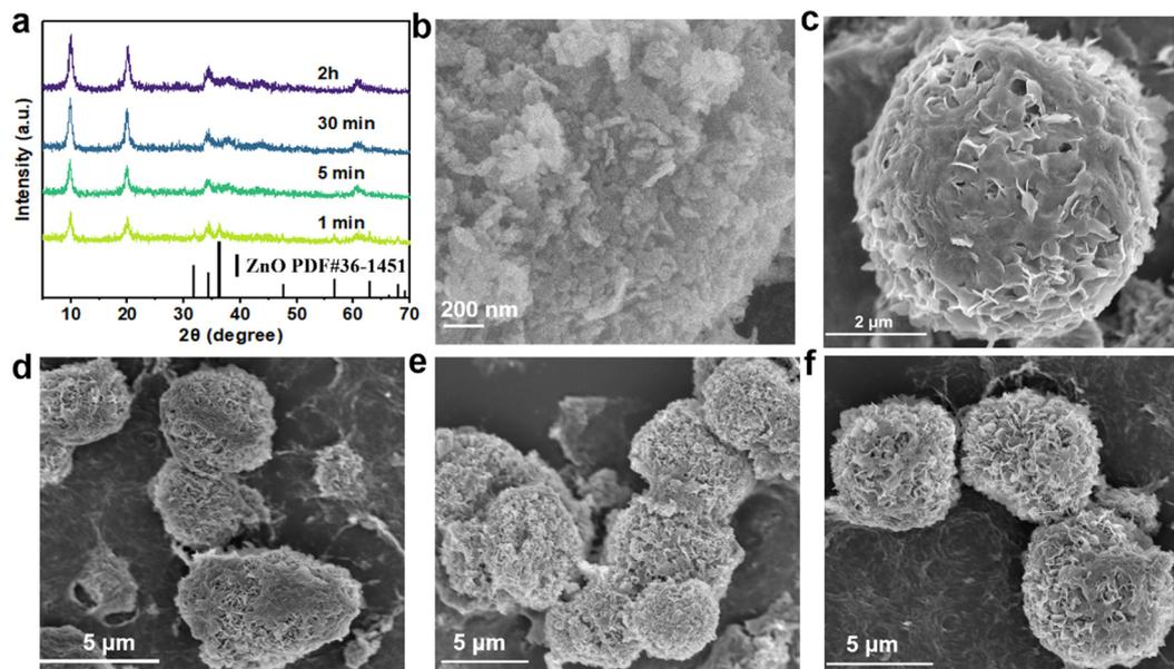
Fig. 2 (a) XRD patterns of samples obtained at different reaction times; (b) SEM image of the ZnO precursor; (c–f) SEM images of the samples obtained at different reaction times ( $t = 1$  min, 5 min, 30 min, and 2 hours, respectively).
