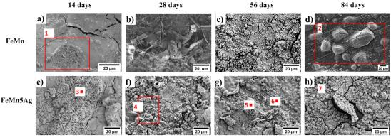
Fig. 3 Top-view SEM images of the degraded surface of FeMn (a-d) and FeMn-5Ag (e-h) incubated for 14 (a and e), 28 (b and f), 56 (c and g) and 84 (d and h) days in HBSS. (EDS analysis on the highlighted areas and locations is presented in Table 2)
