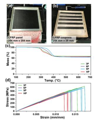
Fig. 4 (a and b) Photos of CFRP composite panel (254 mm × 254 mm) prepared and cut (25 mm × 254 mm) for mechanical testing. (c) Thermogravimetric analysis to determine resin-to-fiber ratio after comand processing. (d) Stress-strain curves for CFRP posite cure composites.
