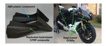
Fig. 9 (left) Photo of a ketal-based CFRP composite replicated from an original ABS motorcycle component and install. Multiple ketal-based CFRP components were installed on the motorcycle shown (right) and have been field tested approximately two years (at time of manuscript submission)
