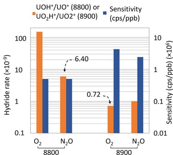
Fig. 2 Comparison of the hydride formation rate and sensitivity with Agilent 8800 ICP-MS/MS (left) from Jaegler *et al.* (2020) and Agilent 8900 ICP-MS/MS (right) using  $\text{O}_2$  or  $\text{N}_2\text{O}$  as a reaction gas in the CRC.
