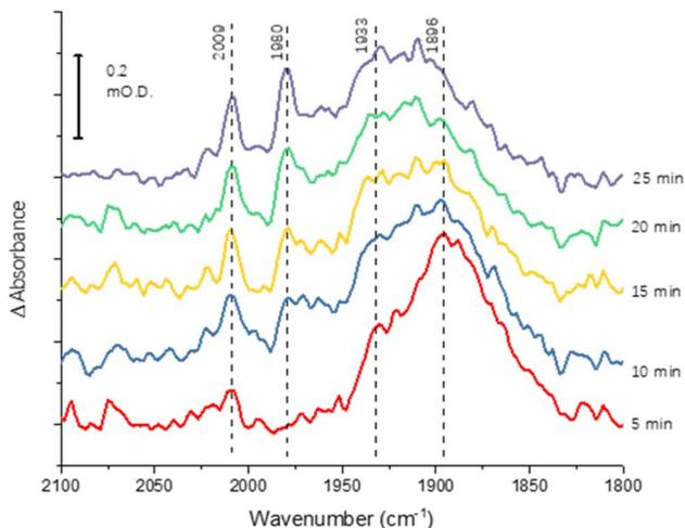
Fig. 4 Time-course spectra for CO binding to nitrogenase MoFe protein at  $-0.9$  V. The protein was covalently attached to the electrode using the carbodiimide coupling reaction. Spectra are calculated from a background at  $-0.7$  V, recorded prior to the step to  $-0.9$  V.
