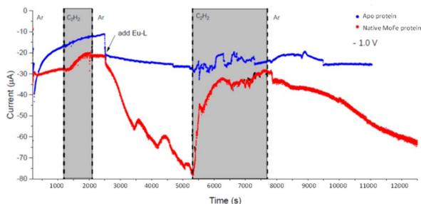
Fig. 5 Electrochemical experiment at  $-1.0$  V examining the effect of  $C_2H_2$  on electrocatalytic proton reduction by nitrogenase MoFe protein and apo protein. At the commencement of the experiment, the buffer flowing through the cell contained no Eu-L mixture, but Eu-L was introduced at 2500 s. The buffer in the solution reservoir was flushed with Ar, except in the periods marked in grey, when  $C_2H_2$  was flushed through the solution reservoir.
