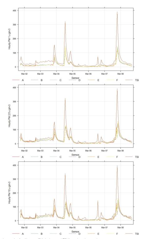
Fig. 3 Hourly average time series for AltasensePM devices and TSI for colocation week
