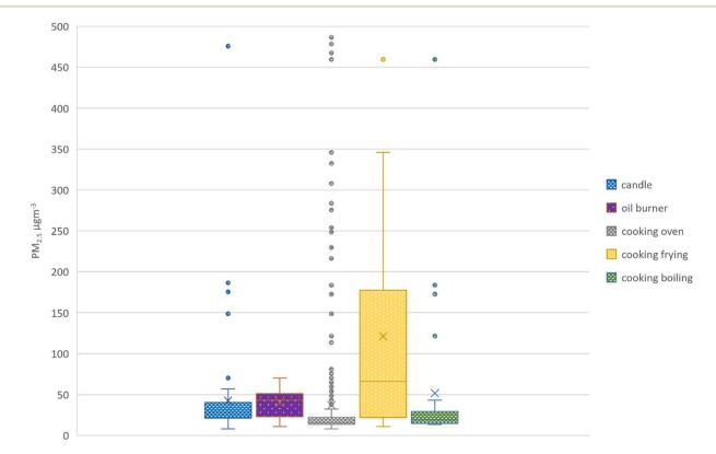
Fig. 8 Distribution of PM<sub>2.5</sub> concentrations in living room during various activities. Cooking occurred in the adjoining kitchen whilst oil burner and candle were located within the living room itself.
