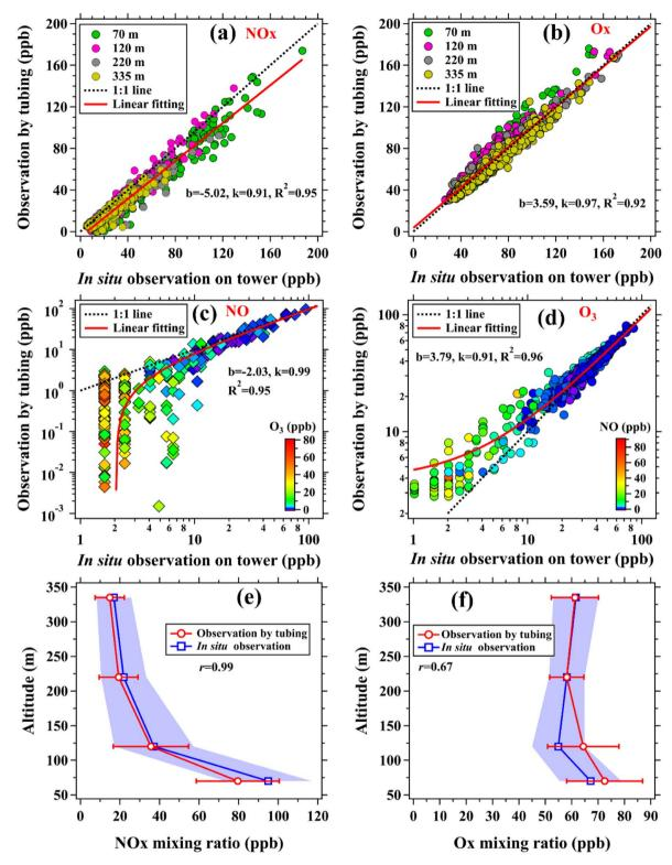
Fig. 6 (a-d) Intercomparisons of NOx, Ox, NO, and  $O_3$  mixing ratios (hourly averages) measured by the vertical observation system (long tubing) and tower platforms (in situ observations) from January 8 to January 26, 2021; Solid lines are linear fittings (y = kx + b). (e and f) Intercomparison of mean vertical profiles of NOx and Ox mixing ratios in the nighttime (LT 0:00-06:00) from January 13 to 15, 2021; r is Pearson's correlation coefficient.
