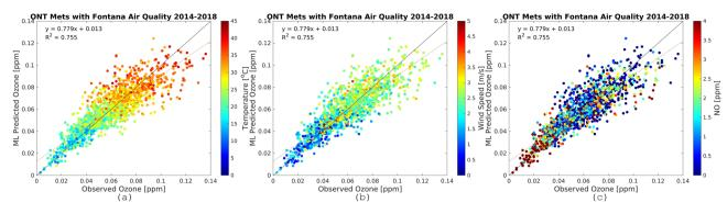
Fig. 8 Observational  $O_3$  (x-axis) and RFR predictions (y-axis) for Fontana air quality and meteorology from the ONT international airport monitoring station. The plots are for the most recent five-year increment from 2014–2018. The color bars show temperature (a), wind speed (b), and NO (c). Plots for other periods are provided in the ESI.†
