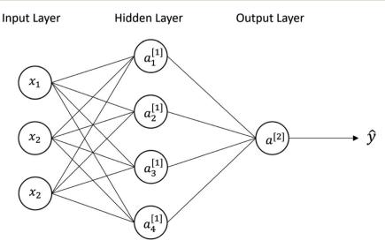
Fig. 4 A fully connected 2-layer neural network diagram with inputs x, four perceptrons in the hidden layer, and one in the output layer.
