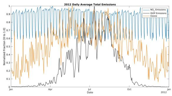
Fig. 14 Daily average NO<sub>v</sub> and isoprene (ISOP) emissions over the model domain normalized by the maximum value in the domain. The periodic oscillation of NO<sub>x</sub> emissions (blue line) is due to weekday/weekend behavior. The black line is the biogenic isoprene emissions in the entire domain. NO<sub>x</sub> and ISOP emissions were extracted from gridded SCAQMD emissions. Twenty-four-hour ozone averages were sampled from the Fontana air monitoring station.
