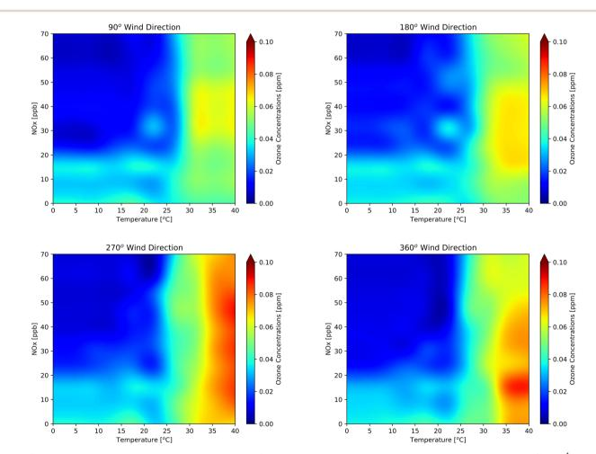
Fig. 9 Contour plots generated by the RFR model trained on ONT meteorology and Fontana air quality at constant wind speed (9 m s<sup>-1</sup>), visibility (16 000 m), dynamic pressure, dynamic relative humidity, and for four discrete wind directions: (a) 90°, (b) 180°, (c) 270°, and (d) 360°.
