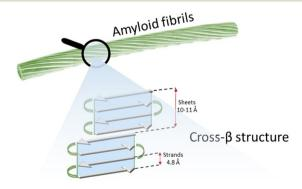
Fig. 1 Schematic representation of the structure of an amyloid fibril, formed by several protofilaments showing a cross- $\beta$  structure.
