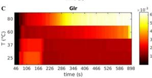
Fig. 3 Bivariate mesh of the integrated SAXS intensity as a function of time and temperature for each carboxylate molecule used. (A) Cit, (B) CitOH, and (C) Glr.
