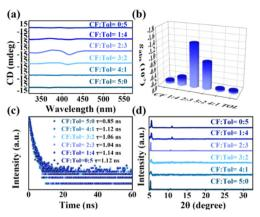
Fig. 3 (a) CD spectra, (b)  $g_{\rm abs}$ -factor values at maximum CD peak, (c) TRPL spectra and (d) XRD patterns of 2D double (R-MPEA)<sub>4</sub>AgBiBr<sub>8</sub> perovskites synthesized at different volume ratios of chloroform (CF)/toluene (Tol).
