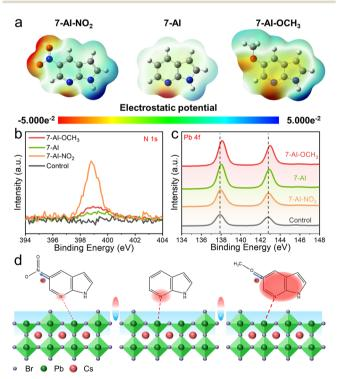
Fig. 1 (a) Molecular structures and electrostatic potential maps of 5nitro-7-azaindole (7-AI-NO<sub>2</sub>), 7-azaindole (7-AI), and 5-methoxy-7azaindole (7-AI-OCH<sub>3</sub>). XPS spectra of (b) N 1s and (c) Pb 4f in CsPbBr<sub>3</sub> films without and with organic molecule treatment. (d) Schematic diagram of electron-transfer-induced coulomb force regulation and the N atom passivated uncoordinated Pb2+
