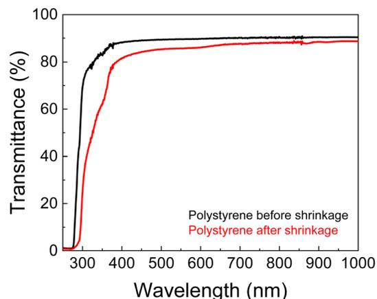
**Fig. 2** Total transmittance UV-Vis-NIR spectra of PS sheets, before and after shrinkage process. The presented spectra are the median of three independent measures.
