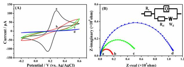
**Fig. 6** Cyclic voltammograms (A) and Nyquist plots (B) of an unmodified GCE (a),  $[(\text{CH}_3\text{CN})_4\text{Cu}]\text{PF}_6/\text{GCE}$  (b), Taniaphos/GCE (c) and Taniaphos- $\text{Cu}^+$ /GCE (d) in 0.1 M KCl containing 5 mM  $[\text{Fe}(\text{CN})_6]^{4-/3-}$ . Inset of (B): the equivalent circuit, where  $R_s$ ,  $R_{\text{ct}}$ ,  $W_d$  and  $Q$  represent the solution resistance, charge transfer resistance, Warburg resistance and constant phase elements, respectively.
