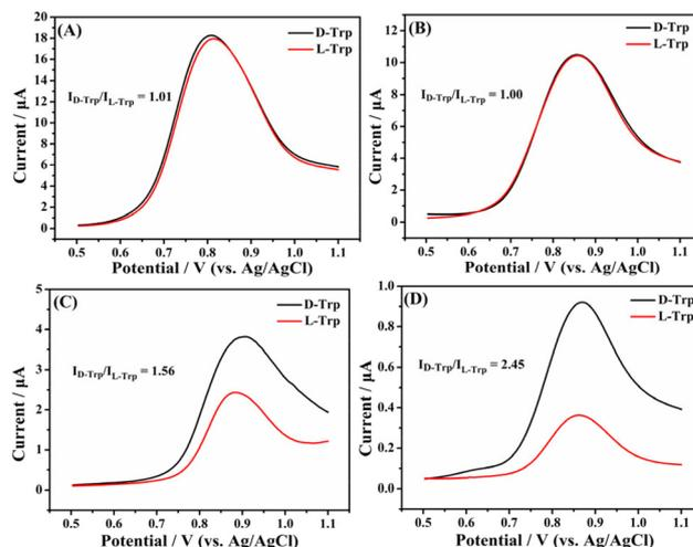
**Fig. 7** Differential pulse voltammograms of an unmodified GCE (A),  $[(\text{CH}_3\text{CN})_4\text{Cu}]\text{PF}_6/\text{GCE}$  (B), Taniaphos/GCE (C) and Taniaphos- $\text{Cu}^+$ /GCE (D) after incubation in 0.1 M PBS containing 1.0 mM L-Trp and D-Trp.
