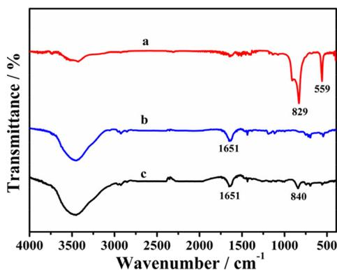
Fig. 4 FT-IR spectra of [(CH<sub>3</sub>CN)<sub>4</sub>Cu]PF<sub>6</sub> (a), Taniaphos (b) and the Taniaphos-Cu<sup>+</sup> complex (c).
