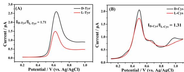
Fig. 11 Differential pulse voltammograms of the Taniaphos-Cu<sup>+</sup>/GCE after incubation in 0.1 M PBS containing 1.0 mM L-/D-Tyr (A) and 1.0 mM L-/D-Cys (B).
