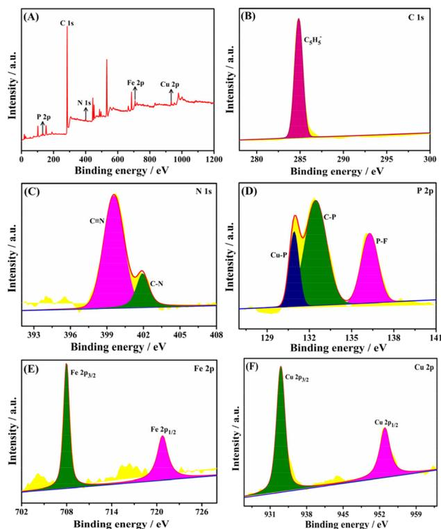
Fig. 5 XPS survey spectra (A) and high-resolution XPS spectra of C 1s (B), N 1s (C), P 2p (D), Fe 2p (E) and Cu 2p (F) of the Taniaphos-Cu<sup>+</sup> complex.
