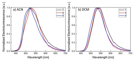
Fig. 6 Normalized electroluminescence spectra of LEC devices ITO/PEDOT:PSS/iTMC:IL(4:1)/Al, (iTMC: 7 (black), 8 (red) and 9 (blue)) with the active layer prepared from solutions in ACN (a) and DCM (b)
