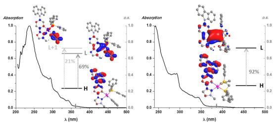
Fig. 3 UV-Vis absorption spectra, S<sub>1</sub> calculated transitions in CH<sub>2</sub>Cl<sub>2</sub> (bars) and molecular orbital plots (isovalue 0.03) of compounds 5 (left) and 7 (right).
