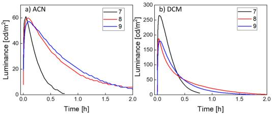
Fig. 5 Time-dependence of the luminance [cd m<sup>-2</sup>] of LECs ITO/PEDOT:PSS/iTMC:IL(4:1)/Al, (iTMC: **7** (black), **8** (red) and **9** (blue)) with the active layer prepared from solutions in ACN (a) and DCM (b). All the devices shown were driven with a pulsed current with an average current density of 50 A m<sup>-2</sup>.
