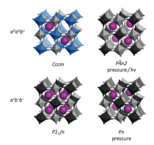
Fig. 5 Tilted structures of Rb-based PBAs. (a)  $Rb_{0.90}Cu[Co(CN)_6]_{0.92}$ , where the tilting is driven by Jahn–Teller distorted Cu (blue) and the unusual Rb arrangement; <sup>26</sup> (b)  $Rb_{0.97}Mn[Fe(CN)_6]_{0.99}$  under pressure; <sup>50</sup> (c)  $Rb_2MnMn(CN)_6$  at ambient conditions; <sup>47</sup> and (d)  $Rb_{0.87}Mn[Co(CN)_6]_{0.91}$  under pressure. <sup>49</sup>
