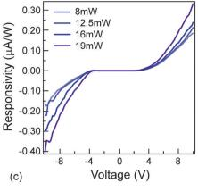
Fig. 5 Photoconductivity of NAI-TPE-PyS. (a) current vs. voltage measurements of the device. Inset: Schematic of NAI-TPE-PyS-coated two-terminal device.  $SiO_2:2 \mu m$ ; Ti: 5 nm; Au: 100 nm. Device channel size: length  $\times$  width = 200  $\mu m \times 5000 \mu m$ . (b) current vs. time measurements of the device at different incident optical powers. (c) Responsivity vs. voltage of the device at different incident optical powers.
