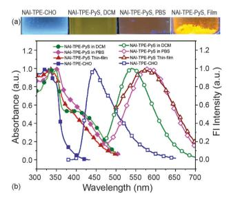
Fig. 4 Optical absorption and emission properties of NAI-TPE-PyS. (a) Images of fluorescence from NAI-TPE-CHO and NAI-TPE-PyS solutions and solid powder ( $\lambda_{\rm ex}$  = 365 nm). (b) Normalized absorption spectra (solid symbols) and emission spectra (hollow symbols) of NAI-TPE-PyS in DCM or PBS or in solid state, and NAI-TPE-CHO at  $\lambda_{ex}$  = 390 nm
