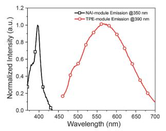
Fig. 3 Emission spectra of NAI-TPE-PyS at  $\lambda_{ex}$  = 350 nm (black squares) and  $\lambda_{ex}$  = 390 nm (red circles) in PBS buffer (concentration: 10  $\mu$ M, containing 1% DMSO).
