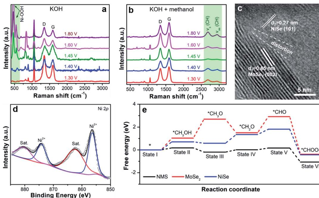
Fig. 4 (a) Potential-dependent Raman scattering spectra of the NMS/CC anode acquired using multiple potential steps in (a) 1.0 M KOH and (b) 1.0 M KOH/1.0 M methanol; (c) HR-TEM image and (d) XPS spectrum of the NMS/CC electrocatalyst after the stability test; (e) calculated MOR free energy profiles.
