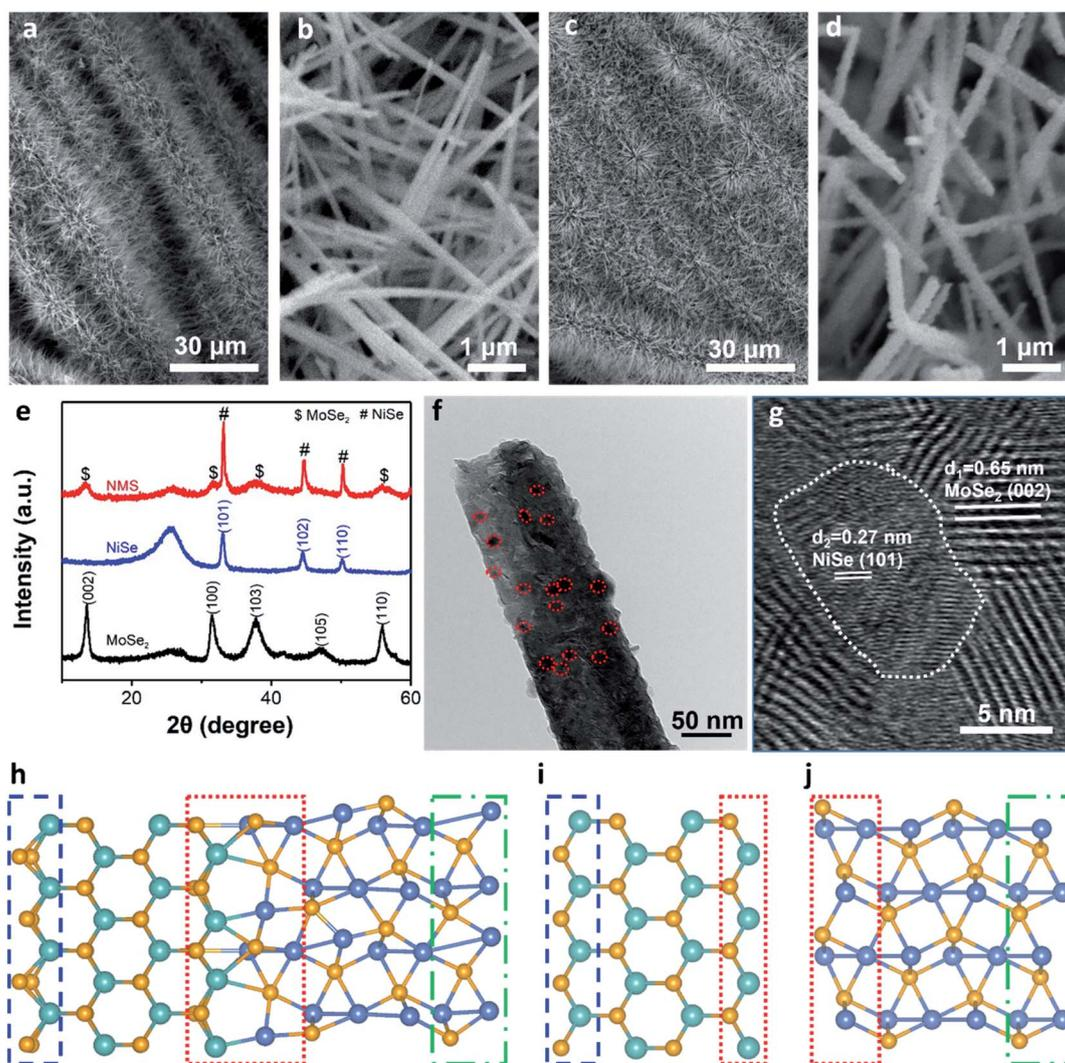
Fig. 1 SEM images of (a and b) NMO/CC and (c and d) NMS/CC; (e) XRD spectra of NMS/CC, NiSe/CC, and MoSe<sub>2</sub>/CC; (f) TEM image (red circles indicate particles anchored on the nanowire) and (g) HR-TEM image of the NMS nanowire. Top view of (h) the simulated NiSe (101)/MoSe<sub>2</sub> (002) heterointerface, and (i) individual MoSe<sub>2</sub> (002) and (j) NiSe (101) surfaces (brown color represents Se, cyan represents Mo, and blue represents Ni).
