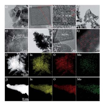
Fig. 1 (a-c) TEM and HRTEM images of In(OH)<sub>3</sub>. (d and e) TEM and HRTEM images of InOOH. (f-h) TEM, HRTEM, and AC HAADF-STEM images of Mo-IOOH/IOH-20. (i and j) The HAADF-STEM image and EDX elemental mappings of Mo-IOOH/IOH-20 with low magnification and high magnification, respectively.
