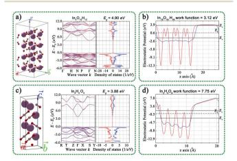
Fig. 6 Geometric structures, band structure, the density of states, and calculated work functions of the (001) surface for (a and b) InOOH and (c and d)  $In(OH)_3$ .
