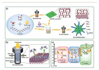
Scheme 1 (a) Synthesis diagrams of Mo modified InOOH/In(OH) $_3$ . (b) Schematic diagram of the CO $_2$  photo-reaction system. (c) The proposed mechanism diagram of photocatalysis under visible-light irradiation ( $\lambda$  > 420 nm).
