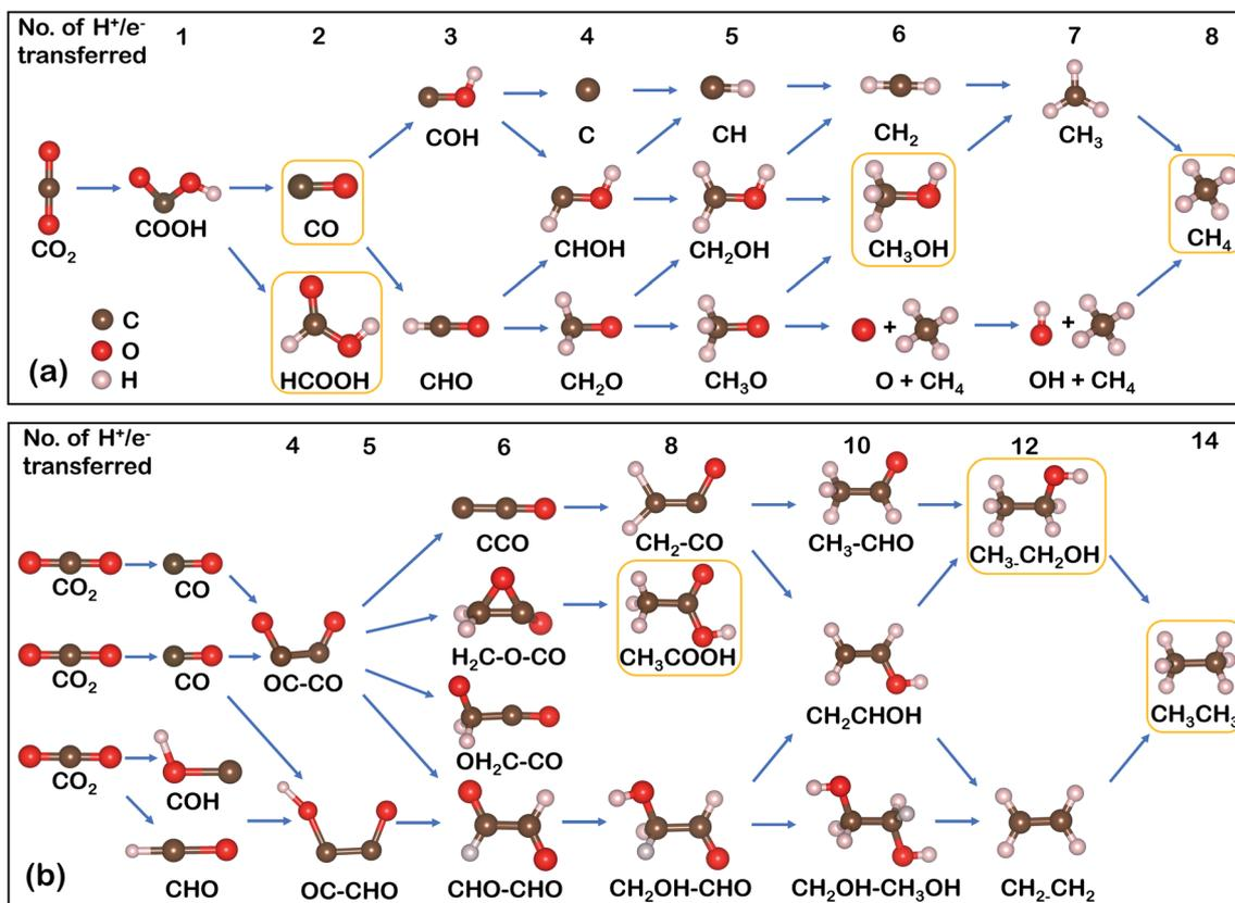
Scheme 1 Overview of possible CO<sub>2</sub>RR roadmaps. The product formation of CO<sub>2</sub>RR on SACs toward various (a) C<sub>1</sub> and (b) C<sub>2</sub> products (main products are boxed) with the number of H<sup>+</sup>/e<sup>-</sup> transferred.
