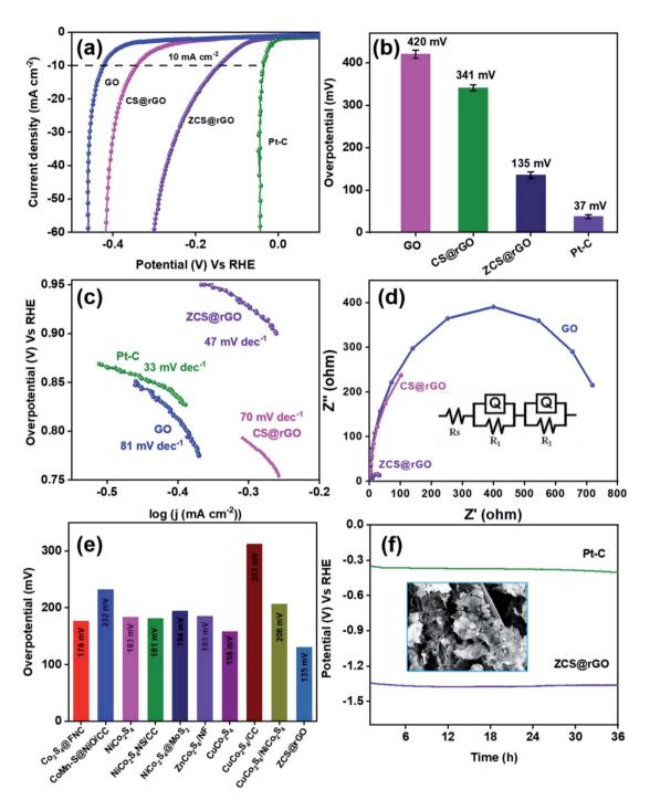
Fig. 4 HER performance. (a) Comparative LSV curves, (b) bar chart exhibiting HER overpotential at  $10 \text{ mA cm}^{-2}$  and (c) Tafel slope of ZCS@rGO, CS@rGO, GO, and Pt-C in 1.0 M KOH. (d) EIS spectrum of ZCS@rGO, CS@rGO, and GO. (e) The comparison of overpotential of ZCS@rGO with recently reported electrocatalysts and (f) long-term chronopotentiometry curves of ZCS@rGO and Pt-C at 10 mA cm<sup>-2</sup>.
