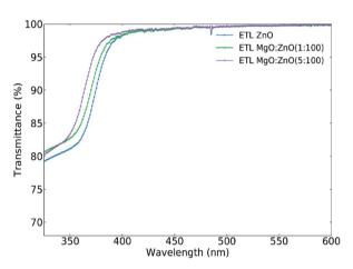
Fig. 3 Transmission spectra of thin films of ZnO and Mg-doped ZnO. There is a blue-shift in the spectrum with increasing Mg-doping
