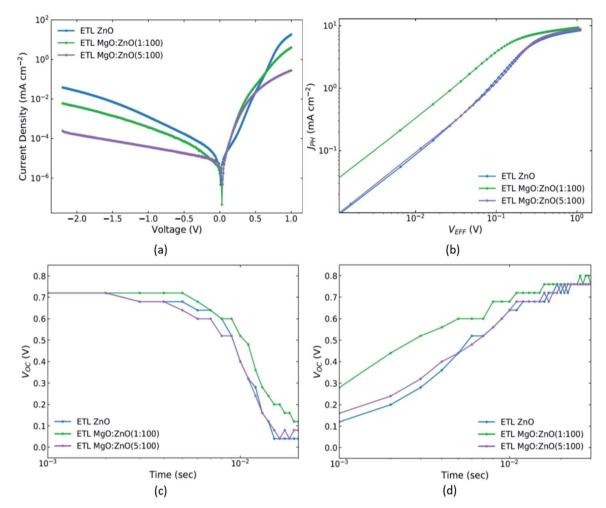
Fig. 4 (a) Current density-voltage curves in the dark. (b) Photocurrent density-effective voltage curves. (c) Open circuit voltage decay curves (in the dark). (d) Open circuit voltage rise curves (under 1 sun).
