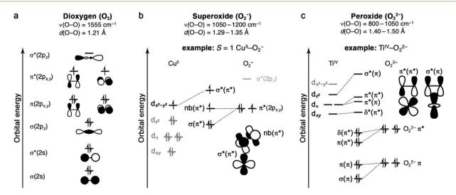
Fig. 1 (a) Qualitative molecular orbital diagram of dioxygen. (b) Qualitative electronic structure of an S=1 end-on  $Cu^{II}-O_2^-$  complex, with key orbital interactions highlighted. (c) Qualitative electronic structure of a side-on  $Ti^{IV}-O_2^{2-}$  complex, showing two molecular orbital interactions. For the resulting molecular orbitals, the bond type is indicated by the nature of the  $M-O_2$  interaction, and the contributing O-O bond type is indicated in parentheses.
