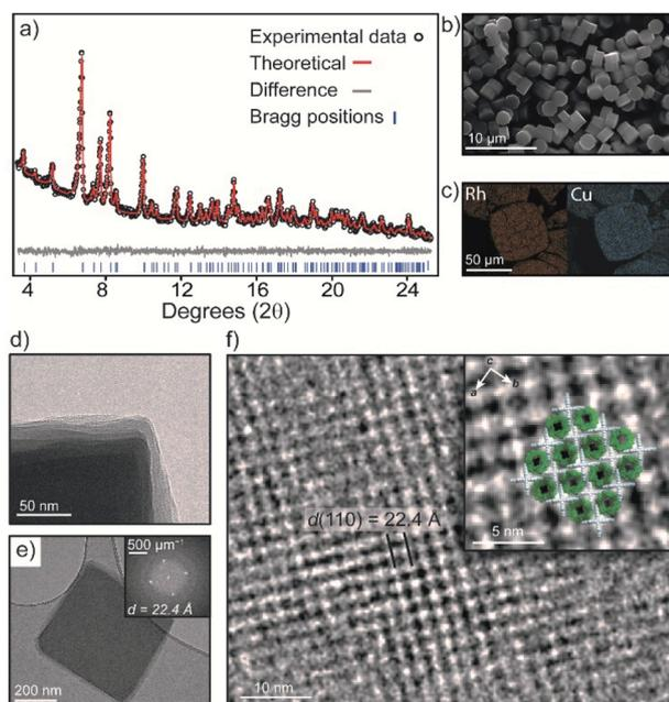
Fig. 3 (a) Rietveld refinement of the PXRD data of **3**; (b) SEM image of **3** obtained from a DMF recrystallization; (c) EDX elemental mapping of Cu and Rh within crystals of **3**; TEM images of **3** (d) the edge of a crystal, showing misalignment of layers; (e) the FFT pattern of a selected crystal; (f) an enlarged image of the same crystal showing the superimposition of the crystal structure of **3** along the *c* axis.
