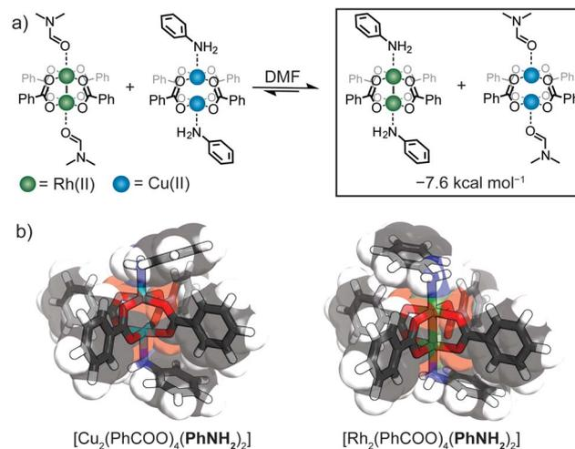
Fig. 5 (a) The ligand exchange reaction between Cu(II) and Rh(III) paddle-wheel complexes as investigated by DFT calculations; (b) a comparison of the optimized structures of  $[Cu_2(PhCOO)_4(PhNH_2)_2]$  and  $[Rh_2(PhCOO)_4(PhNH_2)_2]$ .
