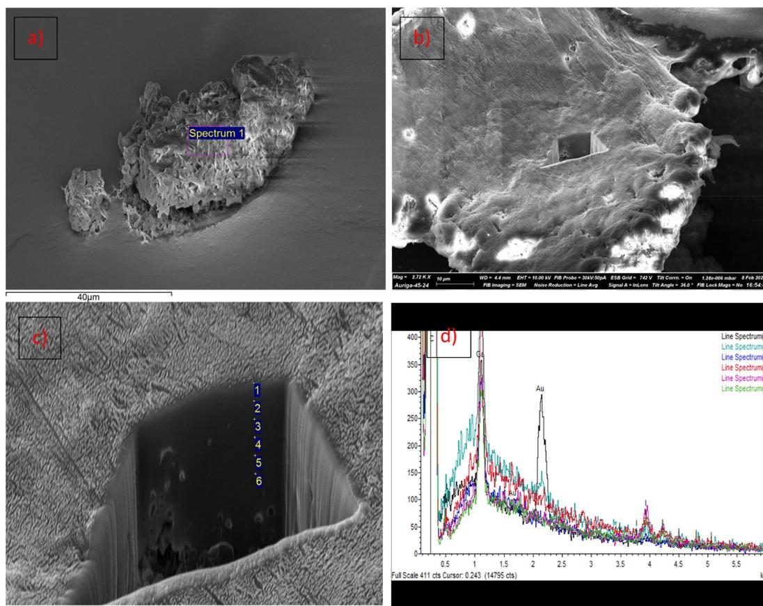
**Fig. 6** (a) SEM image of PE-I/LDPE particle. (b) FIB-SEM image of PE-I/LDPE surface with square hole cut using FIB micro machining. (c) EDX analysis at  $\sim 1 \mu\text{m}$  depth intervals. (d) EDX spectra taken at surface (spectrum 1) and at  $\sim 1 \mu\text{m}$  depth intervals (SEM samples were Au-plated for conductivity).
