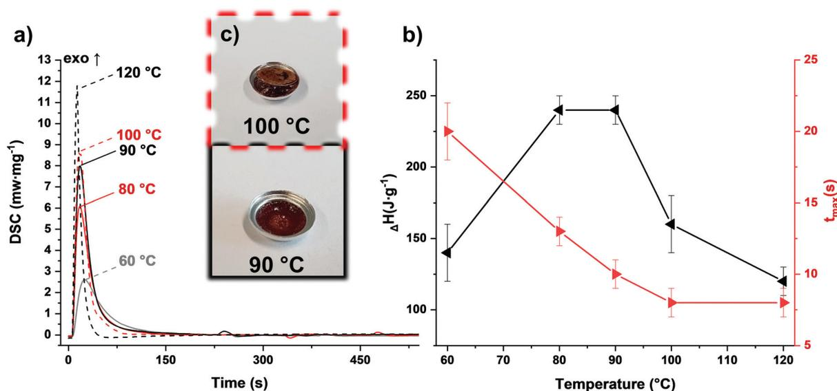
Fig. 3 (a) Photo-DSC of the PF-formulation at 60–120 °C, 2 × 900 s, 320–500 nm, 60 mW cm<sup>-2</sup>. (b) Temperature dependence of photo-DSC results for the PF-formulation: enthalpy change ( $\Delta H$  black) and time until maximal heat is released ( $t_{\max}$  red). (c) Cured Samples at 90 & 100 °C.
