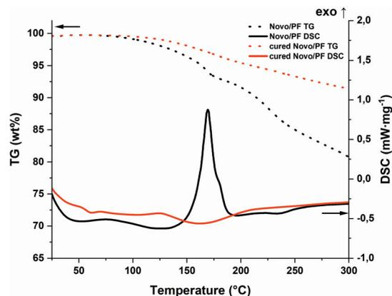
Fig. 4 STA of the PF-formulation (black; TG: dot; DSC: solid) and the photo-DSC cured (red; TG: dot; DSC: solid) sample (90 °C).
