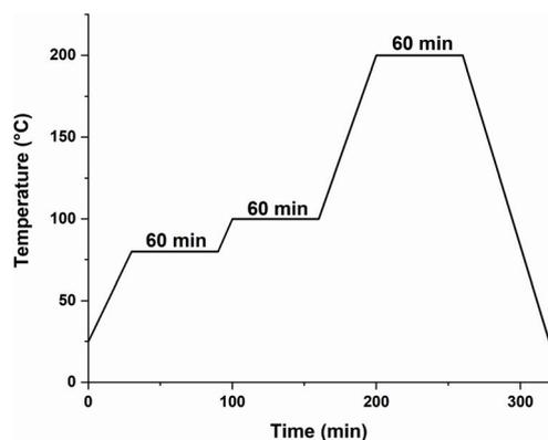
Fig. 1 Post-processing program with a heating rate of 2 K min<sup>-1</sup>.
