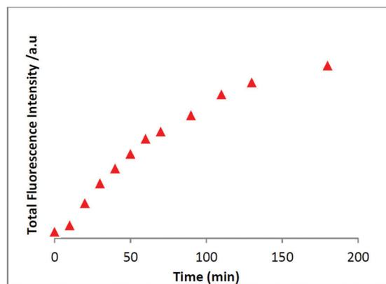
**Fig. 1** Evolution of total fluorescence over time when a polymer decorated with an anthracene chromophore and nitroxide moiety is heated at 100 °C in a degassed solution of toluene containing 2.5 equivalents of AIBN. Figure reproduced with permission from ref. 37. Copyright, Royal Society of Chemistry, 2015.
