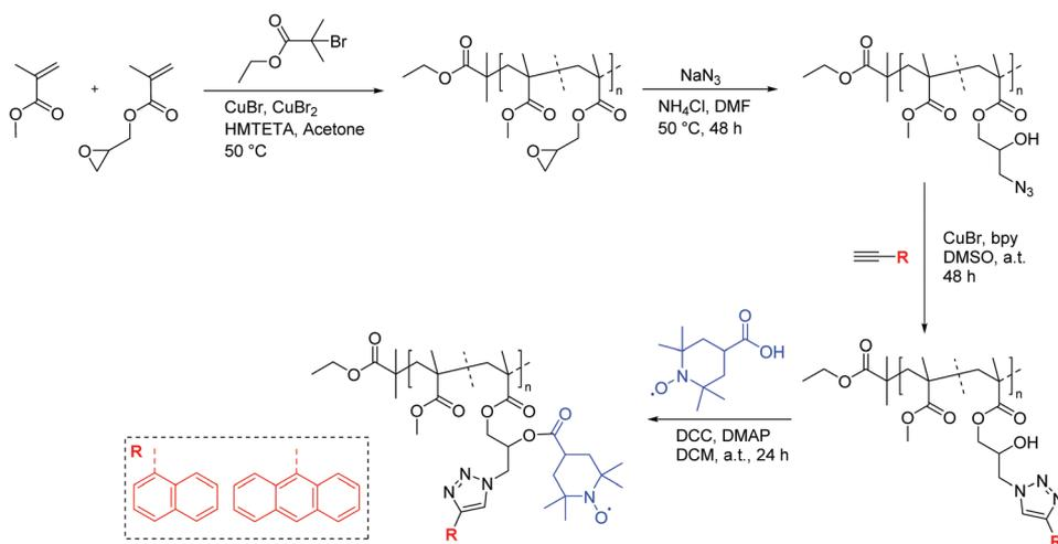
**Scheme 8** Synthetic strategy to obtain profluorescent nitroxide polymers by sequential post-polymerization functionalization reactions (*i.e.*, CuAAC-esterification reactions).<sup>37</sup>
