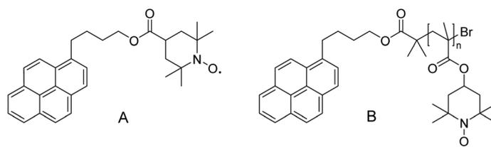
**Scheme 6** Molecular structure of the small-molecule profluorescent nitroxide (A) and macromolecular equivalent (B).<sup>38</sup>
