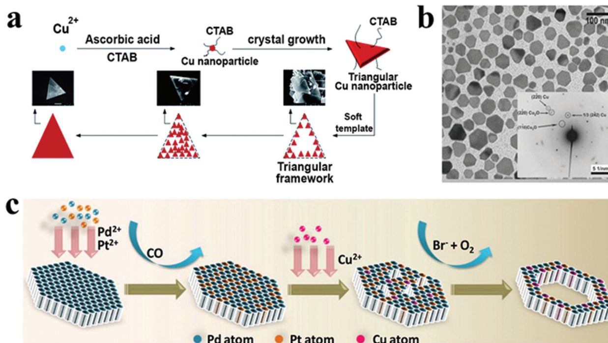
Fig. 10 (a) Schematic illustrating growth mechanism of Cu nanoplates. Reproduced from ref. 138 with permission from RSC, copyright 2017; (b) TEM image of Cu nanoplates synthesized by the reduction of the Cu precursor by hydrazine in DMF using PVP as the stabilizer. Reproduced from ref. 140 with permission from Wiley, copyright 2009; (c) schematic model illustrating the formation of PdPtCu nanorings. Reproduced from ref. 63 with permission from Wiley, copyright 2021.
