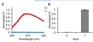
Fig. 2 Buffer logic operation. (A) Symbol of logic gate. (B) Truth table. (C) The normalized fluorescence spectra of logic operation with different inputs. (D) Normalized FI at 471 nm. The concentrations of DCH and BSBOTPE used are 6 µM and 141 µM, respectively. Excitation wavelength was set at 350 nm. n = 3.
