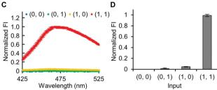
Fig. 3 AND logic operation. (A) Symbol of logic gate. (B) Truth table. (C) The normalized fluorescence spectra of logic operation with different inputs. (D) Normalized FI at 471 nm. The concentrations of DCH and BSBOTPE used are 6 µM and 141 µM, respectively. Excitation wavelength was set at 350 nm. n = 3.
