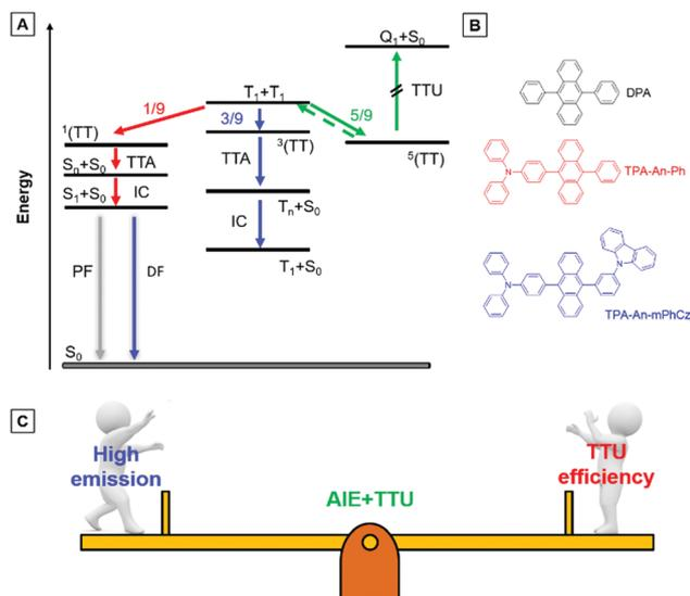
**Fig. 1** (A) Energy-level diagram illustrating the mechanisms of triplet-triplet upconversion (TTU) and triplet-triplet annihilation (TTA).  $^1(TT)$ ,  $^3(TT)$ , and  $^5(TT)$  are the singlet, triplet, and quintet intermediate states.  $S_1$ ,  $T_1$ , and  $S_0$  are singlet excitons, triplet excitons, and ground states.  $S_n$  and  $T_n$  are higher singlet and triplet states. (B) Chemical structures of the anthracene derivatives. (C) Design principle of the blue emitters.
