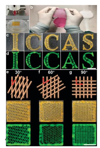
Fig. 3 3D architectures printed from the Gel/Alg/HA/PPV ink. (a) Digital images showing the 3D printing process. (b) The 3D printed large size antibacterial skin patch. (c) Digital and (d) fluorescence images of "ICCAS" letters printed from the Gel/Alg/HA/PPV ink, scale bar: 1 cm. Pattern diagram, digital and fluorescence images of 3D printed structures with (e)  $30^{\circ}$ , (f)  $60^{\circ}$  and (g)  $90^{\circ}$  pore geometry, scale bar: 1 cm.
