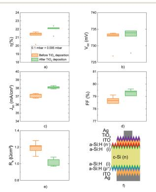
Fig. 8 Statistical distribution of solar cell parameters measured for the devices with the different PLD ITO deposition conditions. (a) Power conversion efficiency, (b) open-circuit voltage ( $V_{oc}$ ), (c) short-circuit density  $(J_{sc})$ , (d) fill factor (FF), and (e) series resistance  $(R_s)$ . Cross-section of the silicon heterojunction cell (SHJ) with a thin ITO and TiO<sub>x</sub> capping layer.
