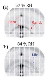
Fig. 5 2-D GI-SAXS patterns of an unoxidised film of the non-deuterated analogue of this proxy at 57% RH (a) and 84% RH (b). The scattering intensities arising from parallel (Para.) and random (Rand.) lamellar orientations are labelled accordingly in the 57% RH pattern. The inverse micellar scattering ring (Mic.) present at 84% RH is also labelled for clarity. The 2-D GI-SAXS patterns are corrected for the incident X-ray intensity and are mapped on the same intensity scale.
