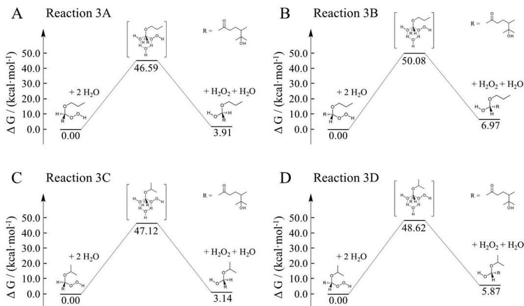
**Fig. 9** Gibbs free energy profiles of water-catalyzed decomposition of  $C_{13}$   $\alpha$ -AHs from  $\alpha$ -terpineol CIs + 1-propanol (A and B) and  $\alpha$ -terpineol CIs + 2-propanol (C and D).
