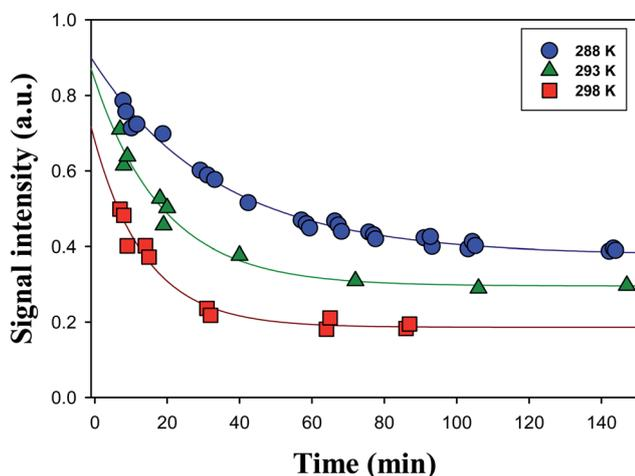
Fig. 3 Decay profiles of the  $\text{Cl}^-$  adducts of the  $\text{C}_{13}$   $\alpha$ -AHs ( $m/z$  297) generated by ozonolysis of  $\alpha$ -Tp (1 mM  $\alpha$ -terpineol, 0.2 mM NaCl) at  $[\text{O}_3]_0 = 0.06$  mM in a 1-propanol : water (1 : 1 = vol/vol) solution at  $T = 288$  K (circles), 293 K (triangles) or 298 K (squares) at pH 4.5 adjusted by 0.05 mM HCl. Lines indicate fittings of signal intensities ( $S$ ) to single-exponential functions with baselines. See the text for details.
