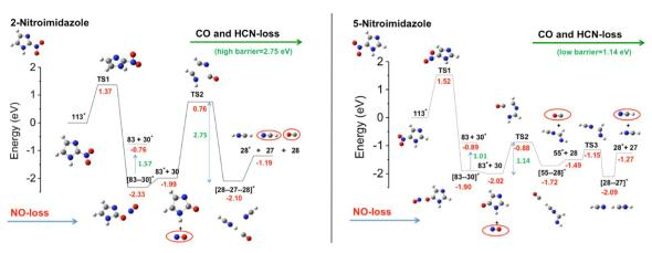
Fig. 11 Potential energy surfaces of the 2NI and 5NI, respectively, for the fragmentation of their corresponding molecular ions  $M^+$  (m/z 113) calculated at the CCSD/6-311++ $G^{**}$ /B3LYP/6-311++ $G^{**}$  level of theory. The molecular ion  $M^+$  as well as the fragments  $[M-O]^+$ ,  $NO_2^+$ ,  $HCN_2^+$ ,  $NO^+$ , and  $HCNH^+$  are all radical ions; the radical symbol • has been omitted for sake of simplicity.
