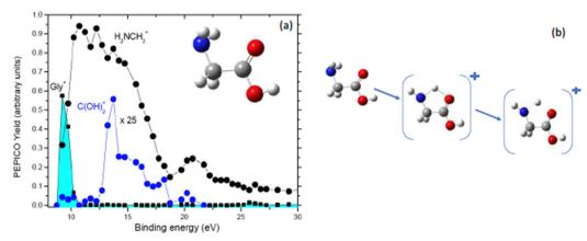
Fig. 7 (a) PEPICO yields of the glycine cation, the  $H_2NCH_2^+$  and  $C(OH)_2^+$  fragments as a function of the binding energy. In the inset the structure of neutral glycine is shown. (b) The proposed mechanism that, via a H transfer in the glycine cation, leads to the formation of C(OH)2+ fragment.
